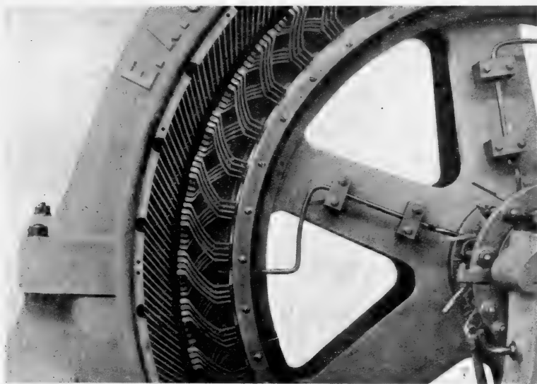
FIG. 265.—Three-phase, Half-coiled, Quadruple-coil, Four-slot Lap Winding. (Bar wound, with separate V-end Connectors.)
